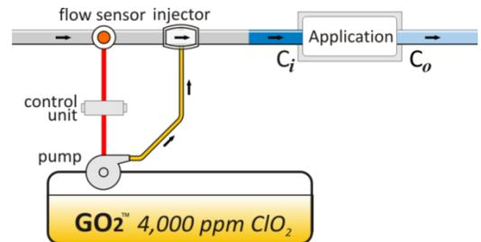
To apply GO<sub>2</sub>, the only equipment required is a storage tank, a flow sensor and dosing pump. These costs are minimal and eliminate the high investment hurdle required by conventional equipment-based ClO<sub>2</sub> generation technology.
