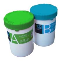
$GO_2$  comes in dry-powder form 1.0kg (2.2 lbs) of component A and 1.0kg of component B produces 50 liters (13.2 gal) of 4,000 ppm chlorine dioxide. Large sizes are available. Only a dosing pump with a flow sensor (optional) and a mixing tank are required.  $GO_2$  is a clean process. It is environmentally friendly and produces zero by-products.
