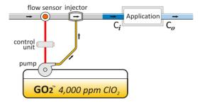
To apply GO<sub>2</sub>, the only equipment required is a storage tank, a flow sensor and dosing pump. These costs are minimal and eliminate the high investment hurdle required by conventional equipment-based CLO<sub>2</sub> generation technology.
